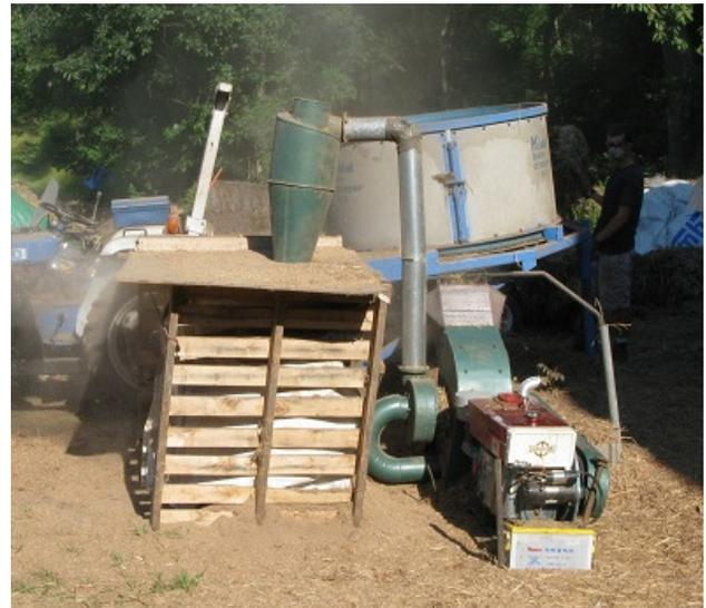
Figure 3. An example of a bale grinder, hammer mill, and dust collection container
