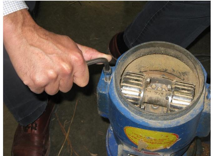
**Figure 5. Some pelletizers have screws to adjust the tightness between the roller and the die**
